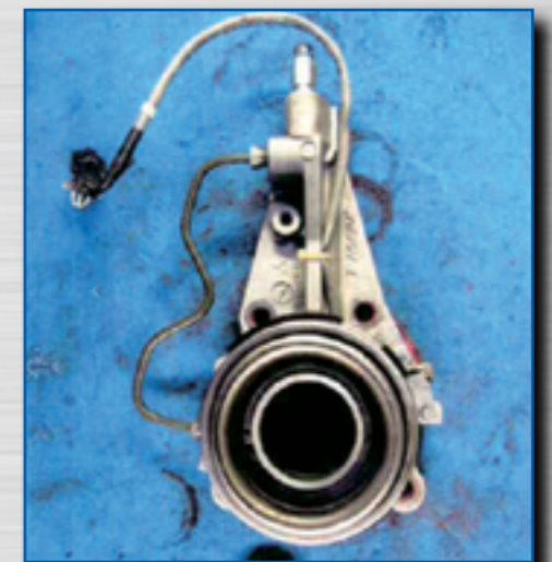
Malfunction of cylinder assembly
