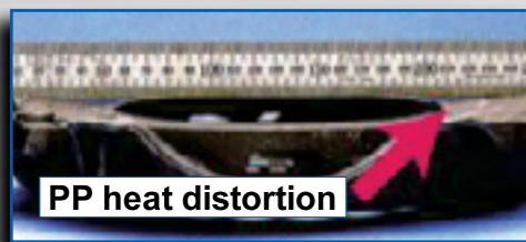
Pressure plate heat distortion
