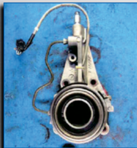
Malfunction of cylinder assembly
