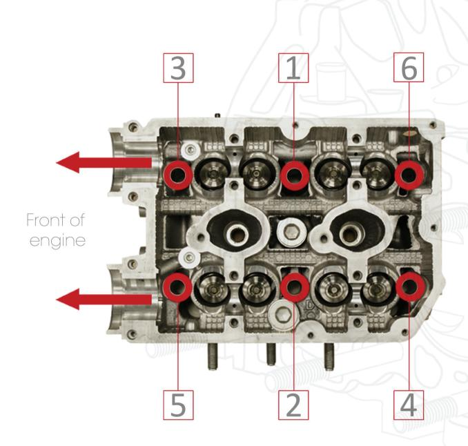
Follow the instructions below for torque settings and be sure to adhere to the diagram opposite, showing the correct tightening sequence.
