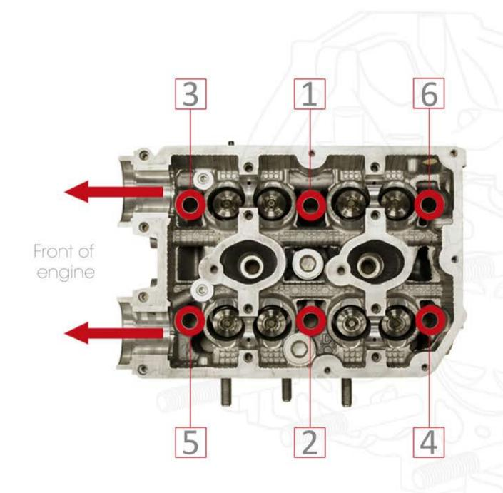
Follow the instructions below for torque settings and be sure to adhere to the diagram opposite, showing the correct tightening sequence.
