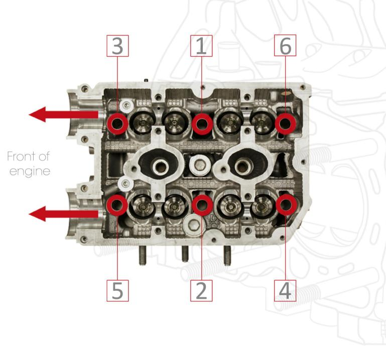
Follow the instructions below for torque settings and be sure to adhere to the diagram opposite, showing the correct tightening sequence.
