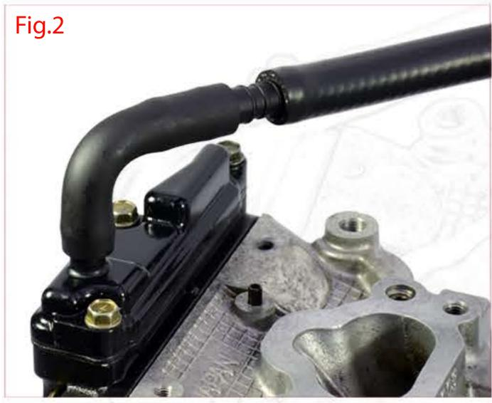
Remove the original breather pipework from the left hand and right hand camshaft covers.
