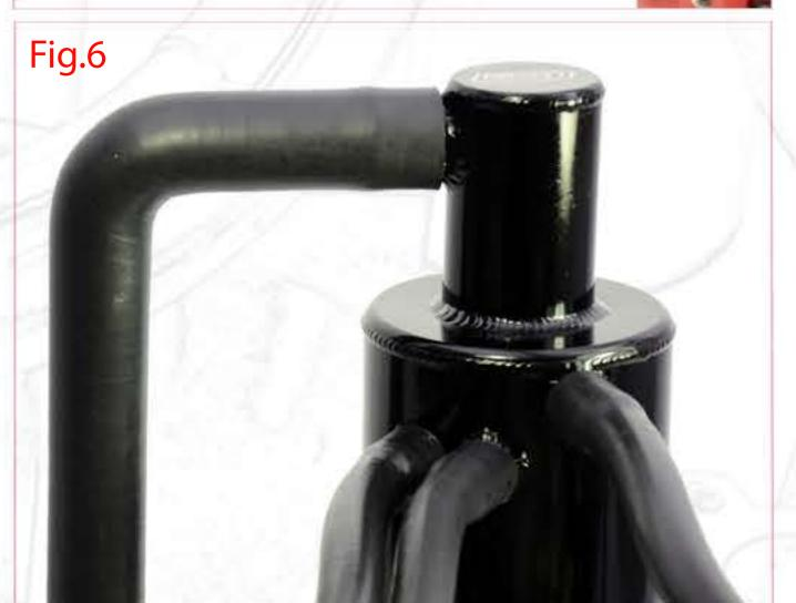
Use the supplied larger 25mm diameter breather hose to vent the catch tank from the top outlet of the tank.
