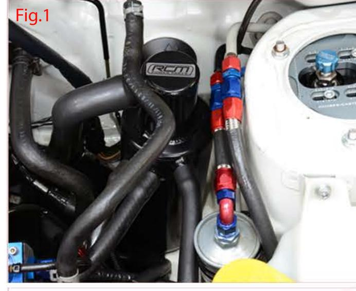
Locate the catch tank on the left hand rear of the chassis leg. Mark the mounting hole locations and drill using a 4.5mm drill bit.
