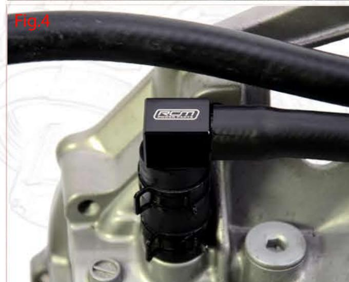
Replace the OE block case breather connector, with the RCM Power Parts connector in Fig 4.
