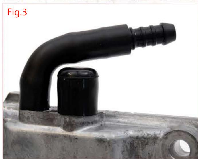
Newage vehicles (2001+) may have 2 breather outlets on the camshaft cover, only the smaller outlet is used.
