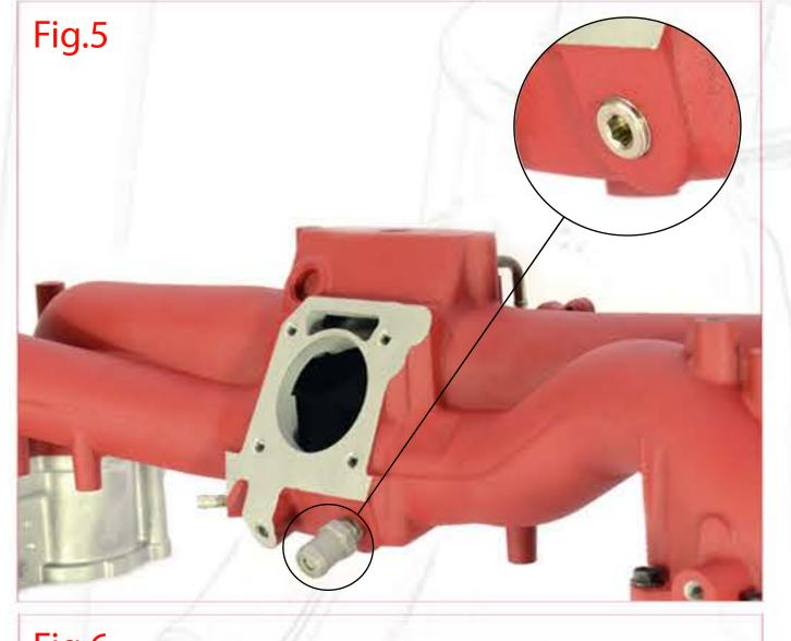
Remove the PCV valve from your inlet manifold and replace with the supplied bung. See Fig.5
